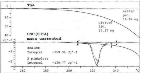
Example: Heat of melting of anthracene in partially open (with evaporation) and in closed pan measured by TGA/SDTA at 5 K/min, 50 ml/min N2. Neglecting the actual mass correction in case of the pierced lid would give a value of 116 J/g only . Lit. value: 161 J/g.
